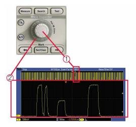
Wave Inspector controls provide unprecedented efficiency in viewing, navigating, and analyzing waveform data. Zip through your 1 Mpoint record by turning the outer pan control (1). Get from the beginning to end in seconds. See something of interest and want to see more details? Just turn the inner zoom control (2).
