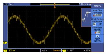
Output of DAC Signal - Notice how FilterVu™ clearly shows the noise-free steps of the DAC in the foreground trace (yellow) which has removed all frequencies above 5.5 kHz. FilterVu also captures and displays high-frequency glitches up to the full bandwidth of the oscilloscope in the background trace (orange).
