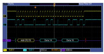
Triggering on a specific data packet going across an  $l^2$  C bus. The yellow waveform is clock and the blue waveform is data. A bus waveform provides decoded packet content including Start, Address, Read/Write, Data, and Stop.
