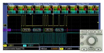
Search -  $l^2C$  decode showing results from a Wave Inspector search for Address value 50. Wave Inspector controls provide unprecedented efficiency in viewing and navigating waveform data.
