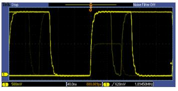
Discover - A waveform capture rate of 5,000 wfm/s maximizes the probability of capturing exclusive glitches and other infrequent events.
